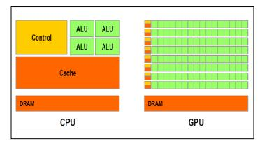
Fig.2: CPU GPU Comparison [3]
